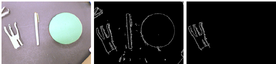
Figure 2. Image pre-processing stages in extracting the boundary of the object Stapler from the original image.
